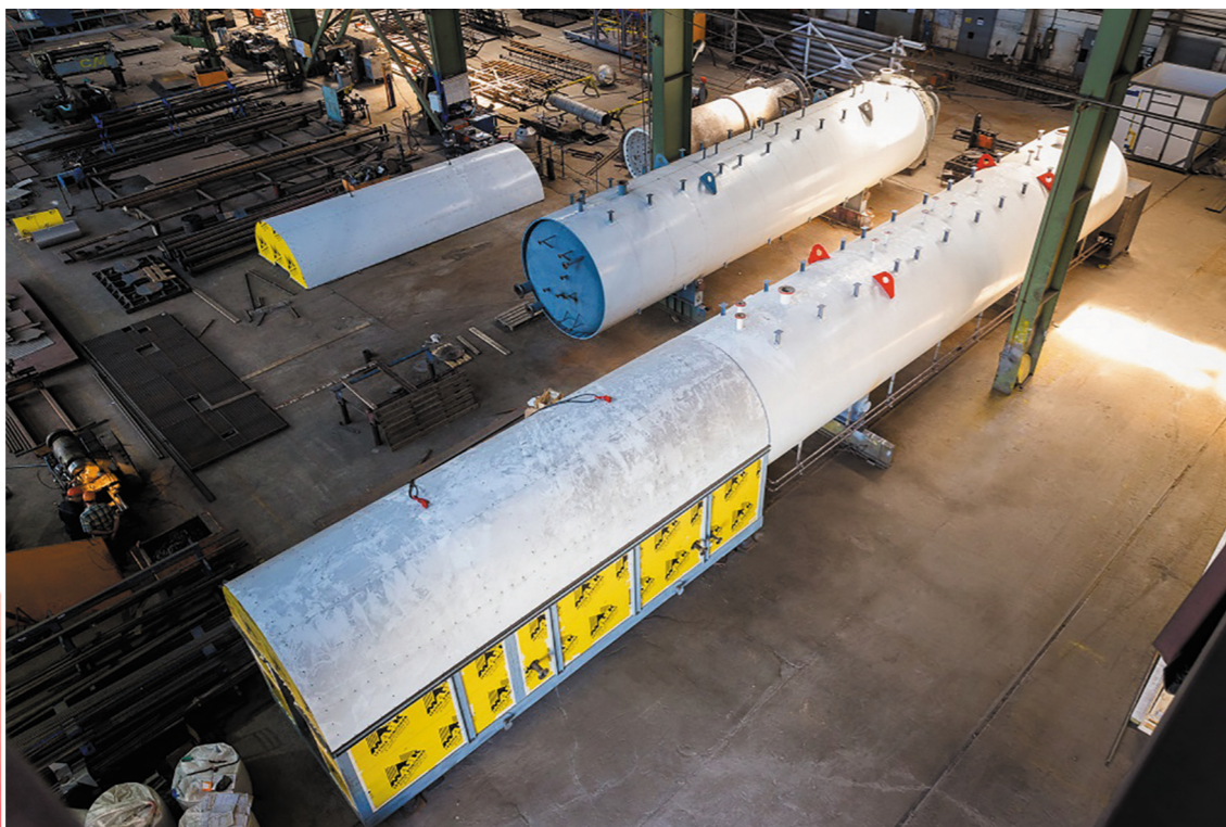
Heater-Treater Oil Treatment Plant
